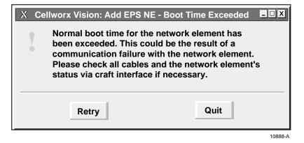
Figure 712-8. Add NE Boot Time Exceeded Window
